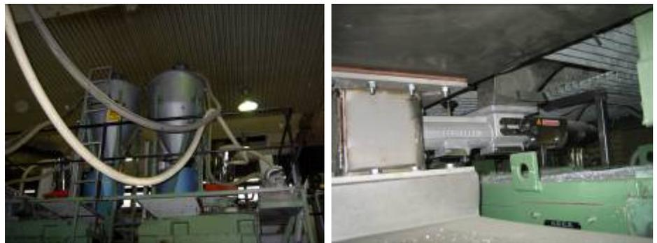
Plastic conveying from silos to the extruders feed hoppers are planned for maximum output 450 kg/h. Conveying is made by vacuum. Choosing of plastic silo will happen so, that you have to move conveying pipe to the wanted silo manually.
